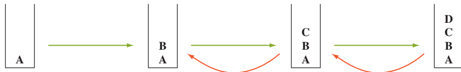
Figure 8.4 A sequence of method calls among the exception throwers. Method D throws an instance of Exception . The green arrows indicate the direction of calls. The red arrows show the reversing of call sequence, looking for a matching catcher. Method B is the catcher in this example. The call sequence is traced by using a stack. (Note: output == System.out .)
