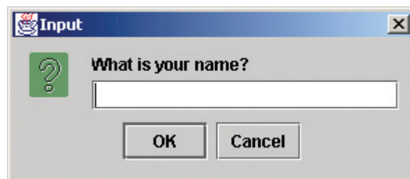
Figure 14.4 An input dialog that appears as a result of calling the showInputDialog class method of the JOptionPane class with “What is your name?” as the method’s second argument.
