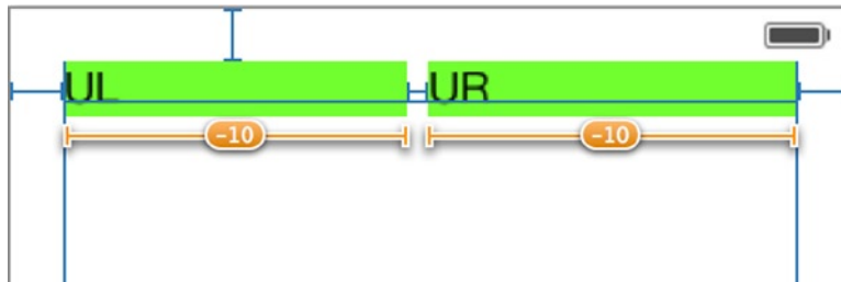
Figure 5-11. The top labels are now made equal in width by a constraint
