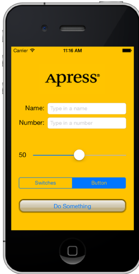
Figure 4-2. Tapping the segmented controller on the left side causes a pair of switches to be displayed. Tapping the right side causes a button to be displayed
