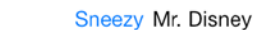
Figure 8-11. The style value 2 does not display the image and places the detail text label in blue letters to the left of the text label
