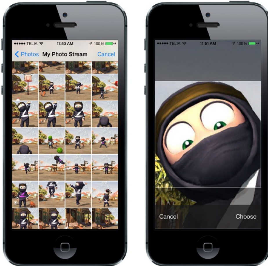
Figure 21-1. An image picker in action. Users are presented with a list of images (left). Once an image is selected, it can be moved and scaled (right). And, yeah, sometimes my camera roll is just pictures of Clumsy Ninja. I blame my children for this
