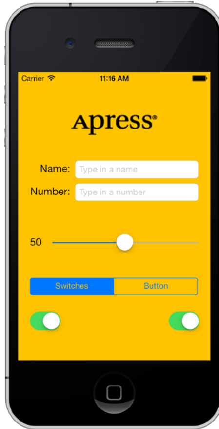
Figure 4-1. The Control Fun application features text fields, labels, a slider, and several other stock iPhone controls
