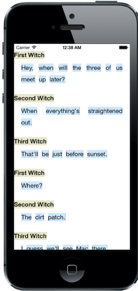
Figure 10-1. Each word is a separate cell. All of this is laid out using a single UICollectionView , and no explicit geometry calculations of our own
