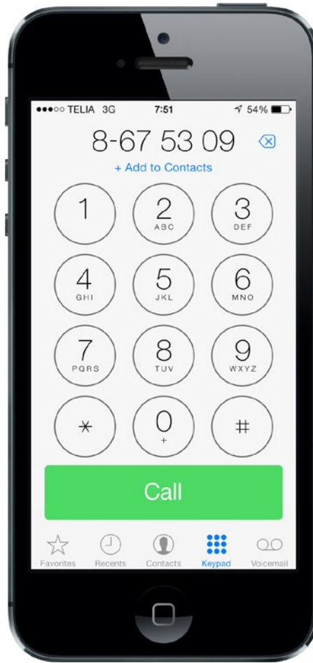
Figure 6-2. The Phone application is an example of a multiview application using a tab bar
