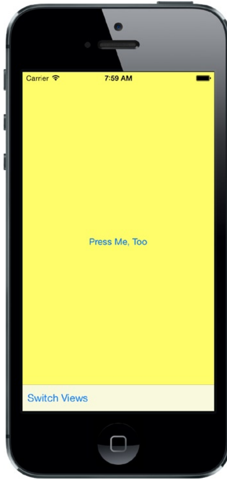
Figure 6-7. When you press the Switch Views button, the blue view flips over to reveal the yellow view
