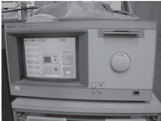
Figure 9-12 A logic analyzer views signals traversing a bus.
