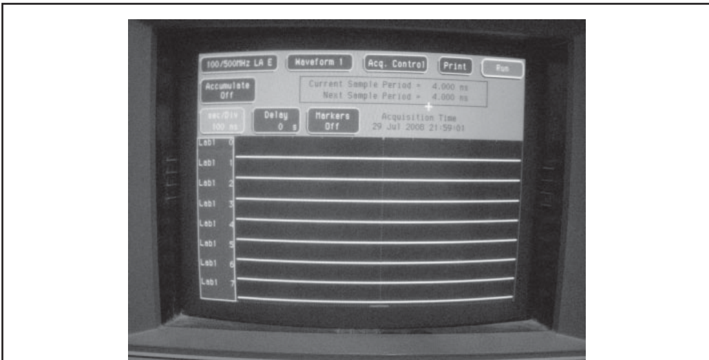
Figure 9-14 A logic analyzer set to receive signals from the attached logic probes
