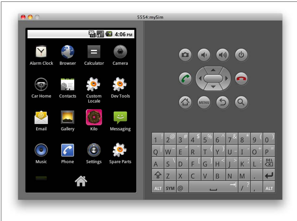
Figure 7-15. You can customize your app's launcher icon by putting a .png file in each of the three drawable directories in your Android project
