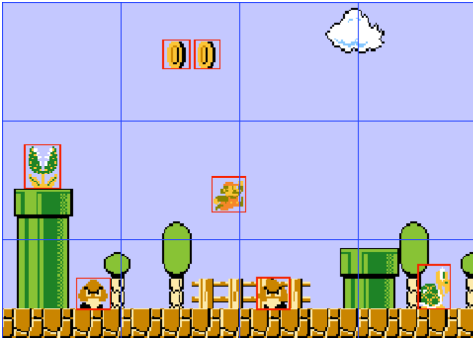
Figure 8–16. Super Mario and his enemies. Boxes around objects are their bounding rectangles; the big boxes make up a grid imposed on the world.
