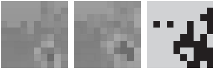
Fig. 17.4. The fitness contest calculation: The filtered patch (center) is “subtracted” from the unfiltered patch (left) — here both patches are false-colored to accentuate gradations occurring within the phenotype. After a threshold has been applied to the magnitude of the difference of the result yielding a bi-level image (right), one point is awarded to the host image for each pixel that is black and one point is awarded to the parasite filter for each pixel that is gray
