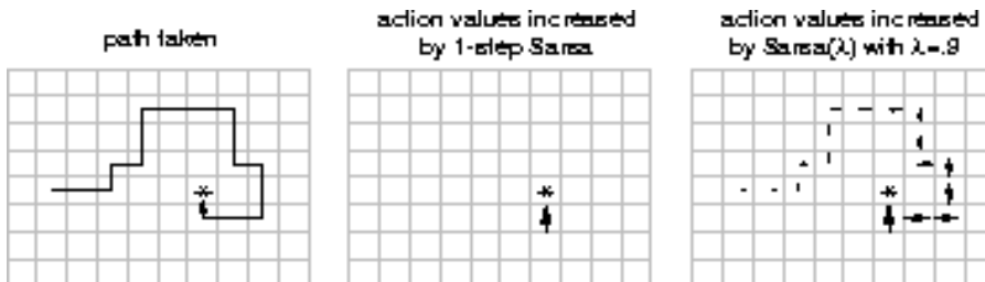
Figure 7.12: Gridworld example of the speedup of policy learning due to the use of eligibility traces. In one episode, 1-step methods strengthen only the last action leading to an unusually high reward, whereas eligibility trace methods can strengthen the whole sequence of actions.
